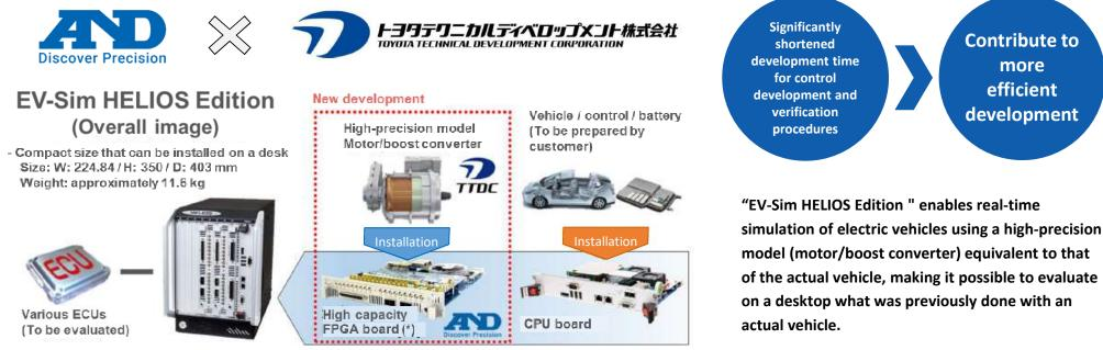
\*FPGA: Abbreviation for Field Programmable Gate Array, an electronic component for digital circuits that can be rewritten any number of times.
